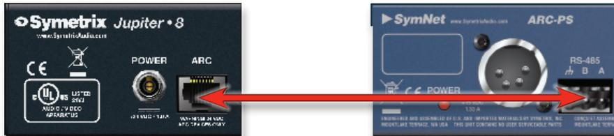
Connecting ARCs to Jupiter hardware is simple using the (RJ-45) ARC port on either the front or back of the device. These ports not only provide communication (RS-485) data, but also +24 VDC power. If the required number of ARCs exceeds the current limits of the Jupiter ARC port(s), an ARC-PS can be used to power additional ARCs. Connecting a Jupiter ARC port to the RS-485 port on the ARC-PS is easily accomplished by following one of two methods.
