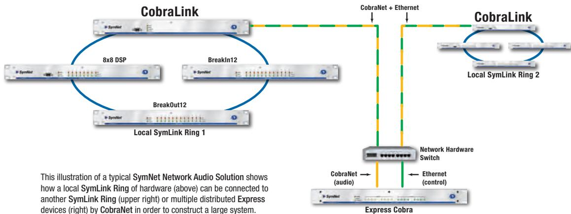
This illustration of a typical SymNet Network Audio Solution shows how a local SymLink Ring of hardware (above) can be connected to another SymLink Ring (upper right) or multiple distributed Express devices (right) by CobraNet in order to construct a large system.
