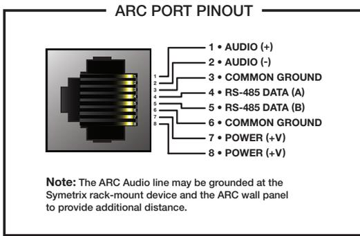
Port Settings: 38.4 kbaud, 8 data bits, 1 stop bit, no parity, no flow control.
